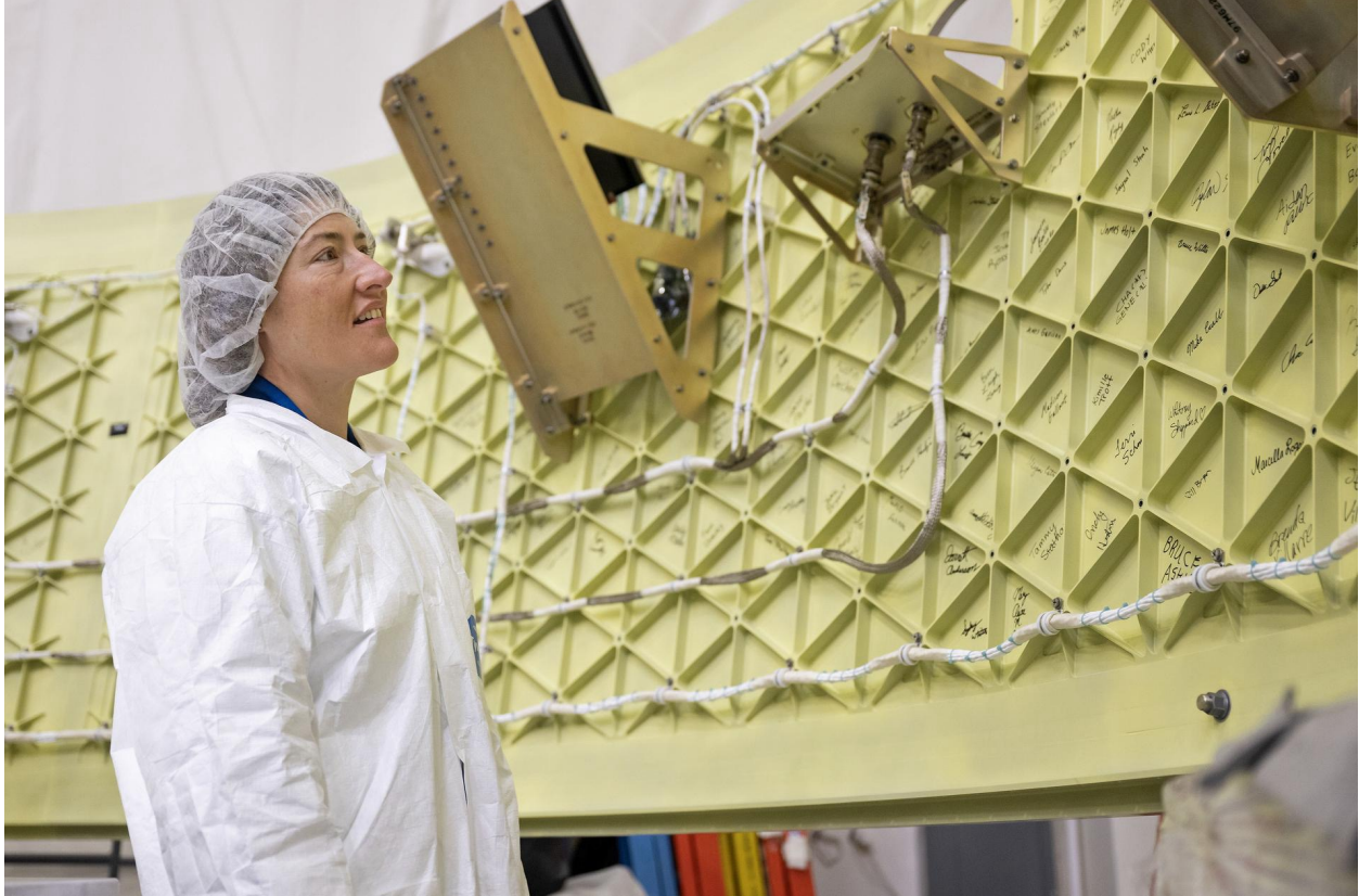
Figure 2-2. Artemis II Astronaut Christina Koch in front of a Secondary Payload Bracket on the OSA.
